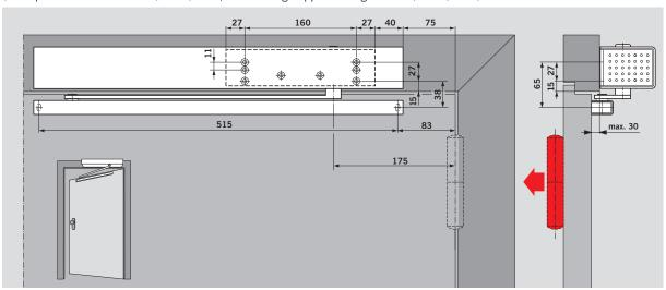
**Plug&Go** Power connector for mains outlet (Example refers to left-hand (ISO 6) door; mirror image applies to right-hand (ISO 5) door)
